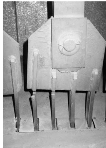
*Figure-4. Grate deformation and fracture of suspension pins after overloading.*
