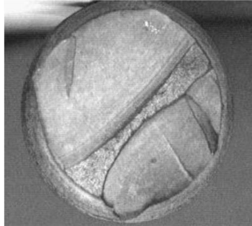
*Figure-3. Fatigue failure of the suspension caused by vibrations.*
