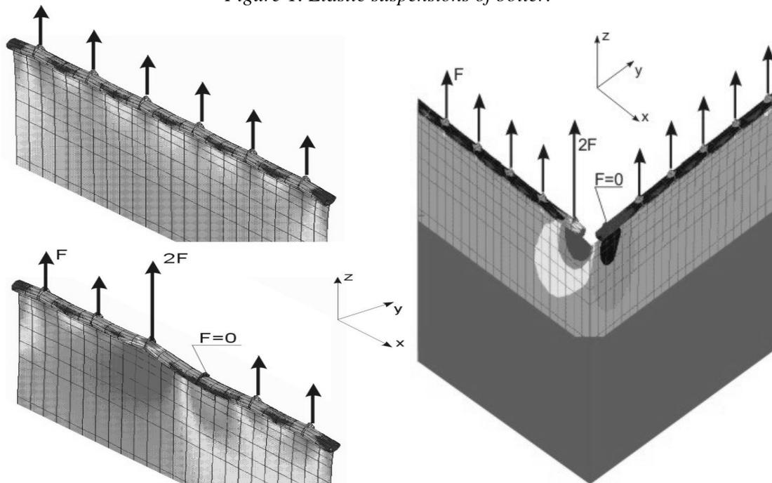
Figure-2. Stress concentration in waterwall caused by suspension overloading and unloading.
